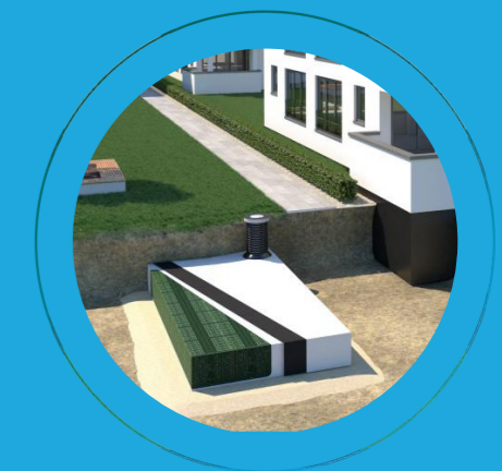
REGENWASSERSPEICHER (Rigolen Systemkonfiguration, Installation)
